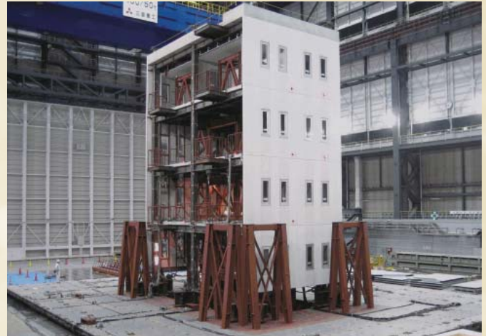
Destructive test of a four-story steel framed structure
