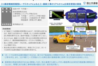
This is an innovative ICT technology that uses a laser scanner mounted on a construction machinery to measure the shape of the finished surface of the roadbed, which is a preliminary process for asphalt-paving, and to process the data in a short period of time to manage the workmanship in 3D.
